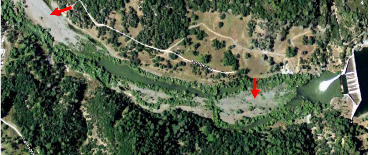
Figure14. The mainstem Eel River riparian zone below Scott Dam has become overgrown due to altered flow patterns and the flood terraces (red arrows) are disconnected as a result. Google Earth map image.
