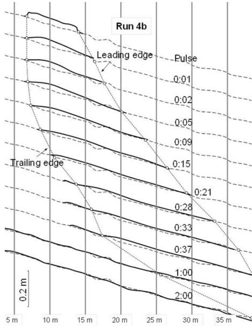
Figure 12. Observed longitudinal profiles of cross-sectionally averaged bed elevation for sand pulse evolution over a gravel-bedded channel. The times are in (hour:min). Figure adapted from Cui et al. (2003b).
